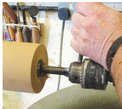
▲ Pic.3 When you have mounted the wood in the chuck you can drill the hole for the tea light. Using a bar in the drill chuck removes any chance of it spinning in the tailstock quill
